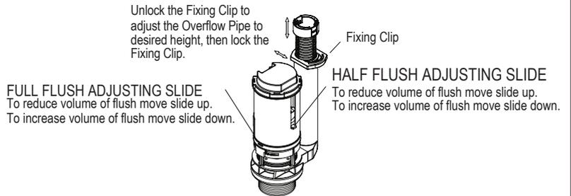
For Cisterns with an Outlet Hole approx 50mm (2") in diameter.
