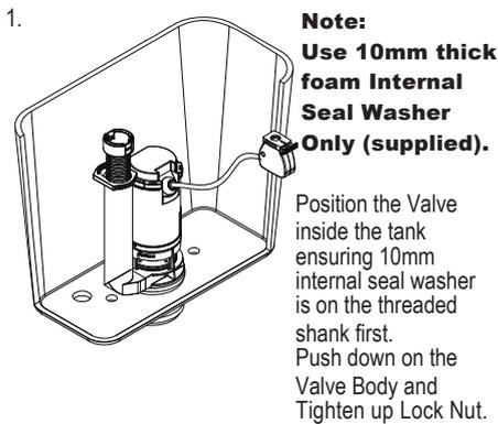
For Cisterns with an Outlet Hole approx 60mm (2.25") in diameter.
