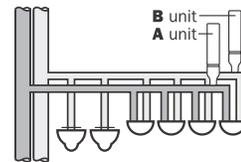
**Arrester Group:** Any ASSE 1010 Certified A, B, C, D, E, or F size arrester. Various connection size and type are for the installer's convenience.
