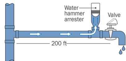
**Fig 2:** Shut-off valve in MIDDLE of long pipe run
