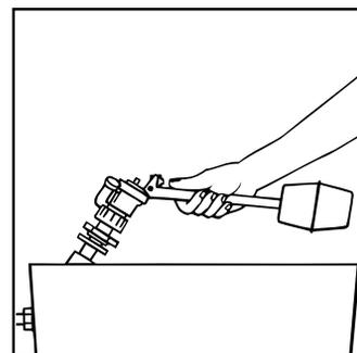
2. Disconnect pipe work and remove old valve.
