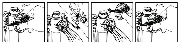
1. Turn off water, flush toilet. Unsnap float rod. Push in on side and remove assembly.
