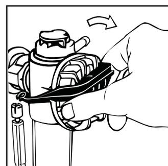
**LOW PRESSURE APPLICATION:** If it takes longer than 4 minutes to refill your cistern, you can increase the flow of water by removing the flow restrictor.
