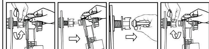
1. Turn off water supply and loosen coupling nut by rotating 1/8 turn until you hear a click.
